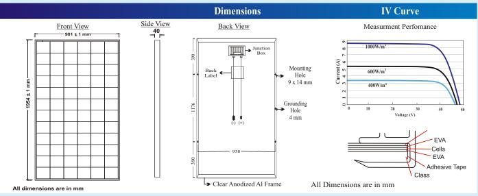
HxWxD 1954 X 981 X 40 mm HxWxD 76.93 X 38.62 X 1.57 inch
