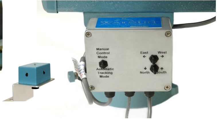
Remote Sun Sensor mounts on the array.
