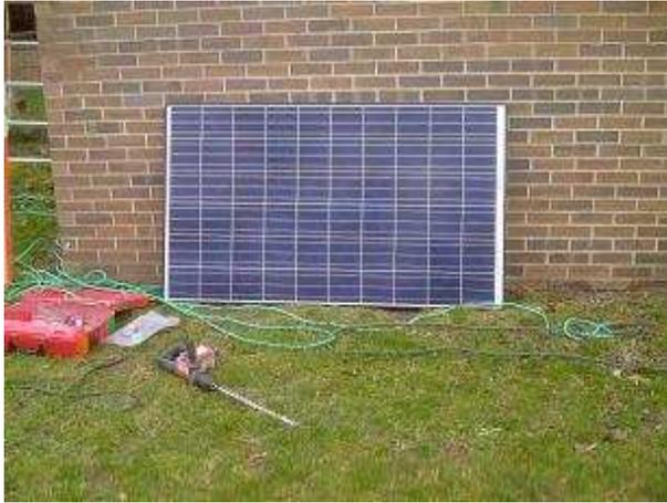
The picture above shows one of the SunModule 240 watt solar photovoltaic panels before it was installed. Five of these panels are mounted on a metal frame and then fastened to the school's south facing wall. The ten panels are wired as two strings of five. This direct current (DC) power then enters the school and is routed to the inverter and connected to the schools electrical system.
